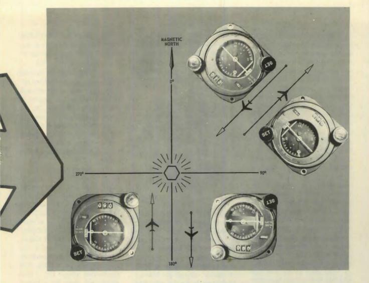
selector knob. It shows the angular relationship between the heading you're flying and the course you've set in the ID-249. If the heading you're flying and the one you've selected are within 90 degrees of each other the pointer will be in the top half of the case. It will show whether you are driving toward, parallel to, or away from your selected radial, regardless of which half of the case it's in. It is good for setting up interception angles but will be inoperative if AC power fails.
